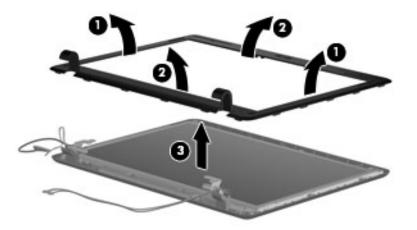
Reverse this procedure to install the display bezel. Be careful to route the cables through the side openings in the hinge covers and avoid pinching the cables between the bezel and display enclosure.
